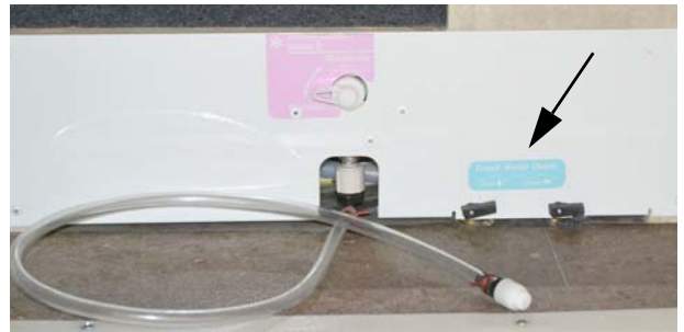
Waterline Drain Valve
