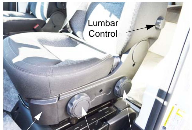
Seat Recline Lumbar Control Front Height Control Rear Height Control Driver Seat -Typical View
