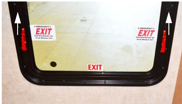
Escape Window (Lift both red safety latch handles UP and push window OUT) -Typical View
