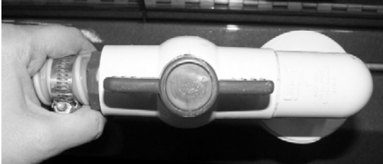
Sewage Drain Hose Valve
