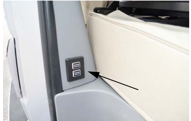
Power Awning Switch (Located near right side of passenger seat) -Typical View
