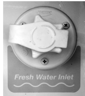
Fresh (City) Water Connection “Fresh Water Inlet” (Located in the water service center)
