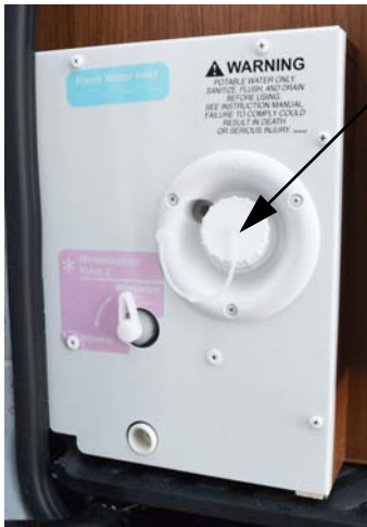
Water Tank Gravity Fill (Located near sliding entrance door) -Typical View
