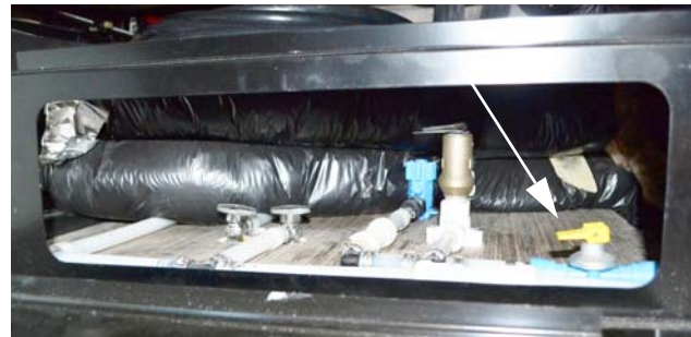
Water Heater Drain Valve (See “Water System Drain Valve Locations” chart at the end of this section for location on your model)
