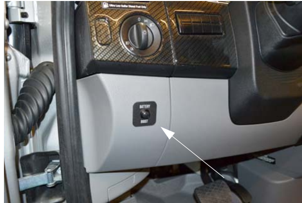
Battery Boost Switch (Located on lower driver side dash)
