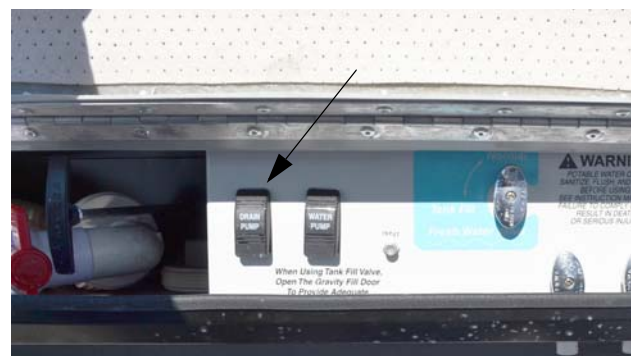
Waste Pump Switch (Located in the water service center)
