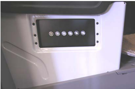
Automotive Chassis 12-Volt Circuit Breakers (Located on outboard side of passenger seat)
