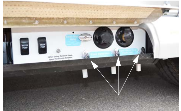
Waterline Drain Valves -Typical installation shown (See the “Water System Drain Valve Locations” chart at the end of this section for locations on your model)
