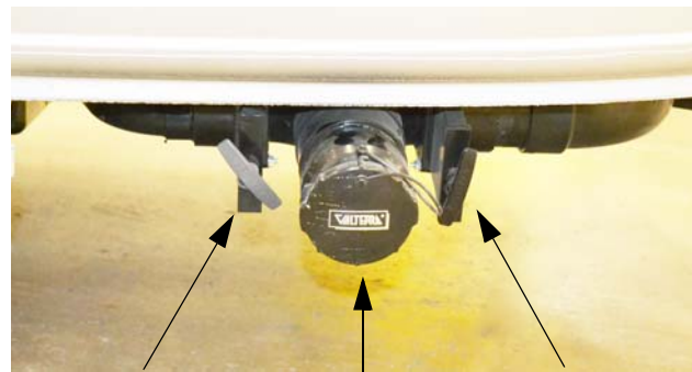
Gray Waste Tank Drain Valve Sewage Drain Outlet Black Waste Tank Drain Valve
