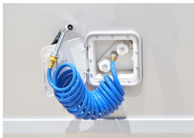
Exterior Shower/Wash Station (Typical)
