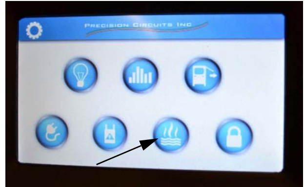
Water Pump Switch
