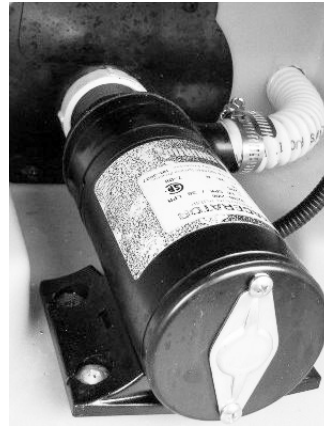
Waste Pump (Located beneath coach) -Typical View
