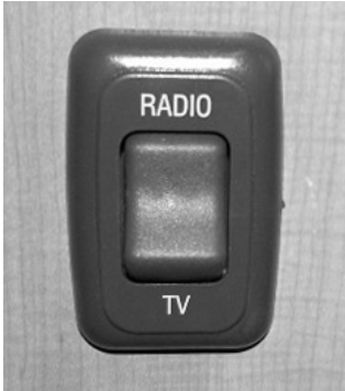
TV/Radio Speaker Selector Switch (Located near exterior TV) -Typical View
