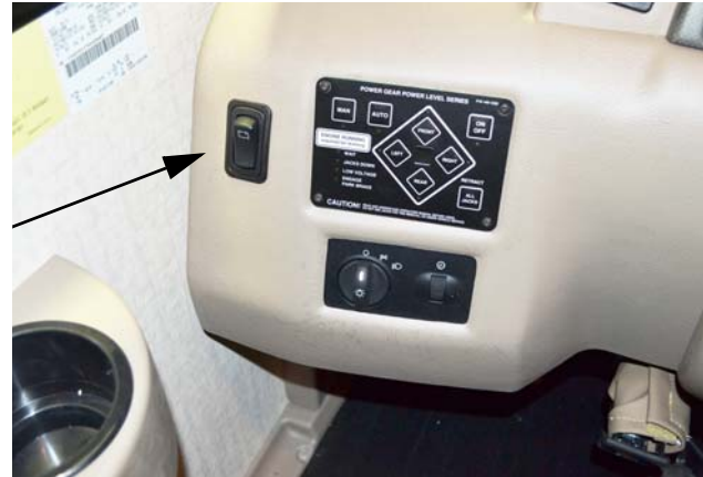
Battery Boost Switch (Located on dash) -Typical View
