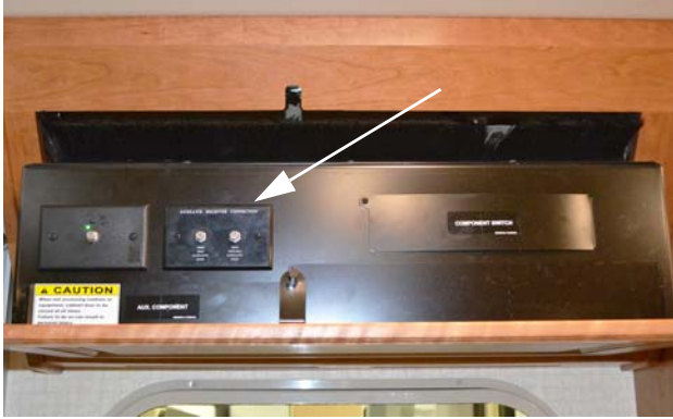
Interior Connection for Satellite Dish -Typical View
