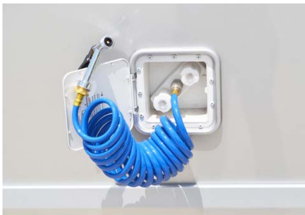
Exterior Shower/Wash Station (Typical)
