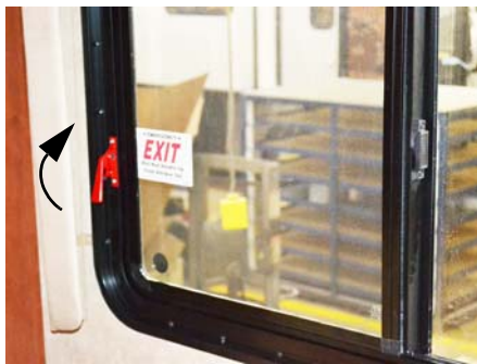
Escape Window (Lift both red safety latch handles UP and push window OUT) -Typical View
