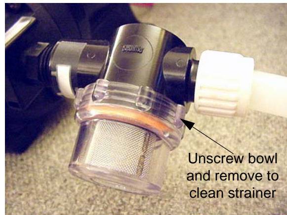
Water Pump Strainer -Typical View
