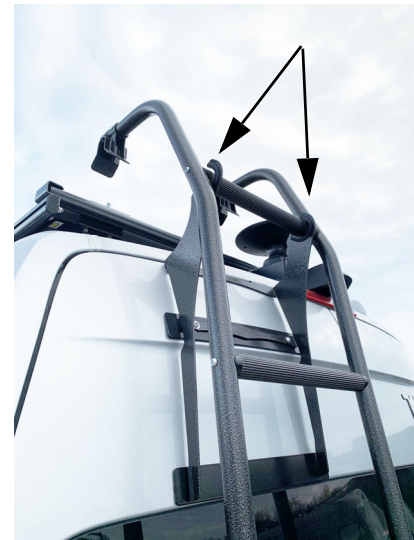
Ladder Storage Rungs -Typical View
