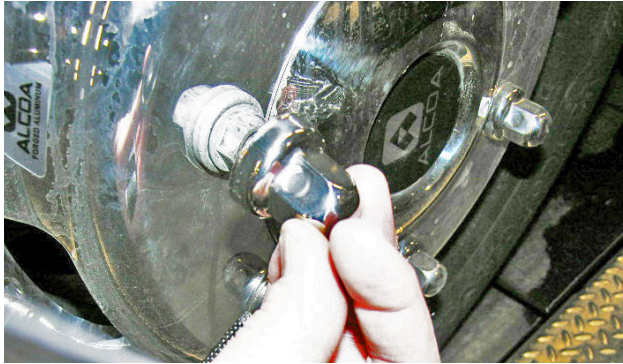
Remove the push on nut covers.
