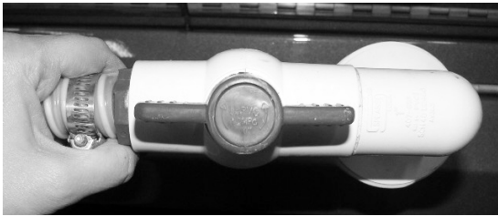
Sewage Drain Hose Valve
