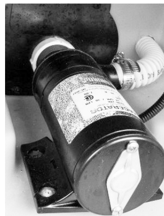
Waste Pump (Located beneath coach) -Typical View
