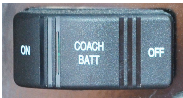
House/Coach Battery Disconnect Switch
