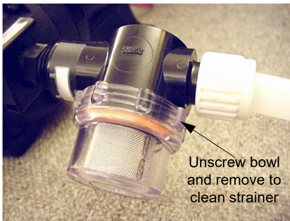
Water Pump Strainer -Typical View
