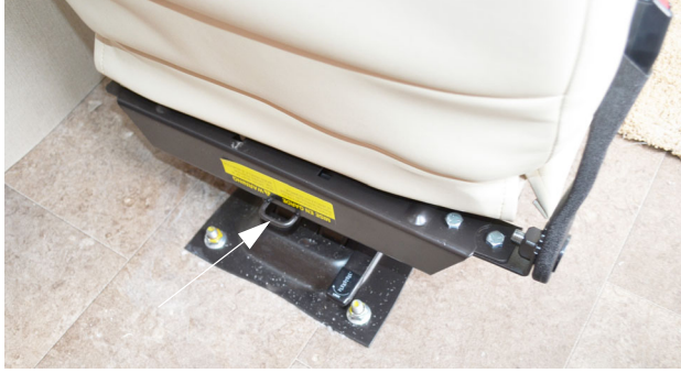
Tether Anchor Loop (Located on back side of companion seat base)
