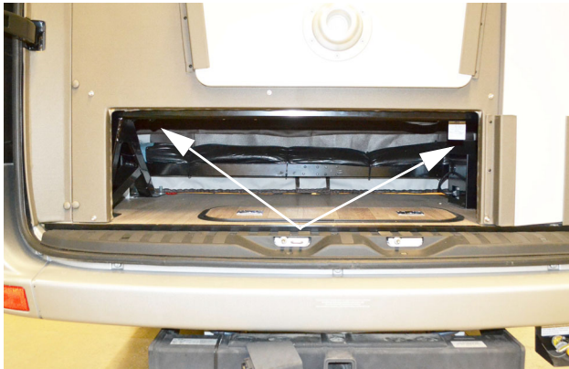
Tether Anchor Loop (Located beneath rear sofa - mounted on frame) *Model 70B
