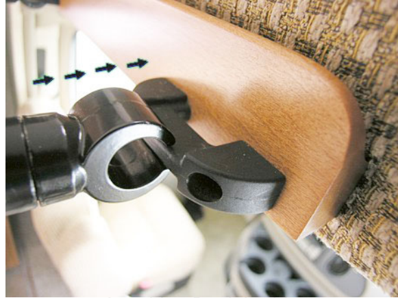
Attaching Bunk Ladder
