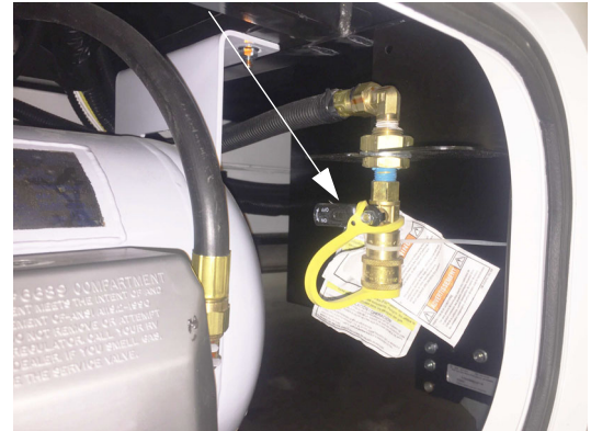
LP Accessory Connection (Located inside propane tank compartment on passenger side of motorhome) -Typical View
