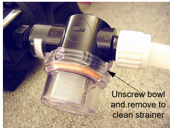
Water Pump Strainer -Typical View
