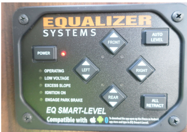
Equalizer Control Panel -Typical View
