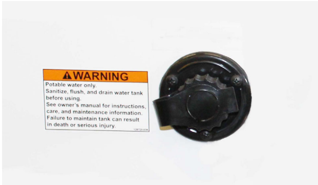
Fresh (City) Water Inlet -Typical View
