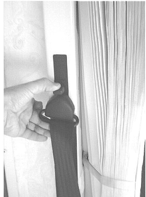
Press lever to adjust shoulder belt height
