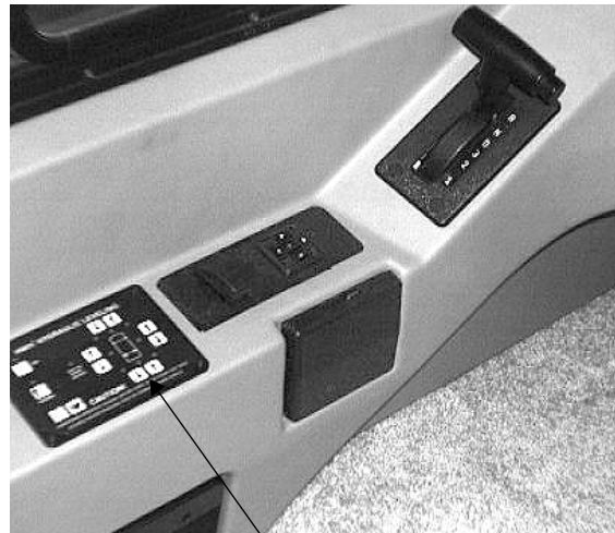
Leveling System Control Panel
