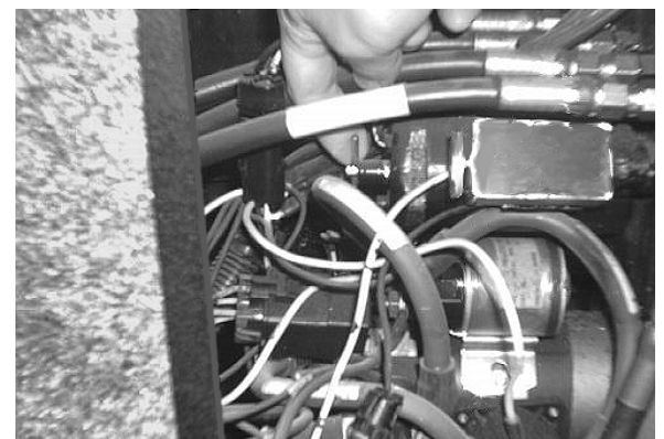
T-Handle valves on forward end of pump
