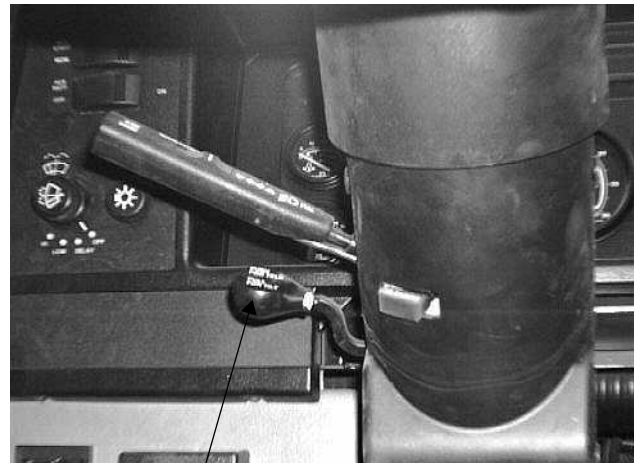
Pull to Tilt Push to Telescope
