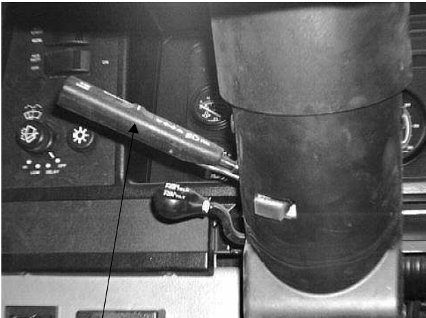
Multifunction Lever Signals/Hi-Lo Beams/Cruise
