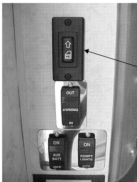
Power Lock Switch (near entry steps)
