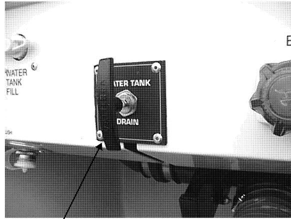
Water Tank Drain Valve (pull to open)
