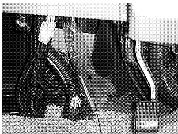
CB Wires (in plastic sheath)
