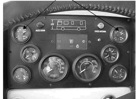
Air Pressure Gauges
