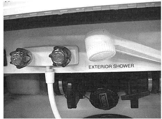
Exterior Shower/Wash Station
