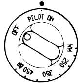
Oven Control Knob in “PILOT ON” position
