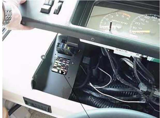
Automotive 12-Volt Fuse Block beneath lift-up dash pod
