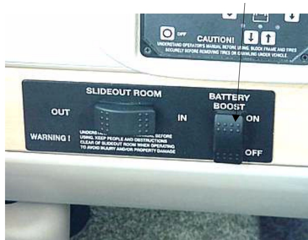
Battery Boost Switch
