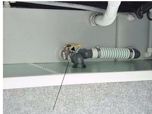
Water Tank Drain Valve in right side compartment toward rear of vehicle
