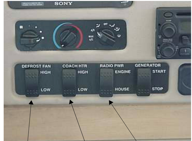
Windshield Defrost Fans Rear Coach Heater Switch Radio Power Switch
