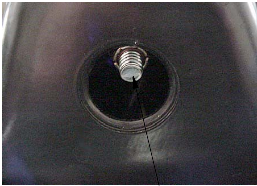
Mirror Arm Pivot Bolt on underside of mounting base. (Shown with access plug removed.)
