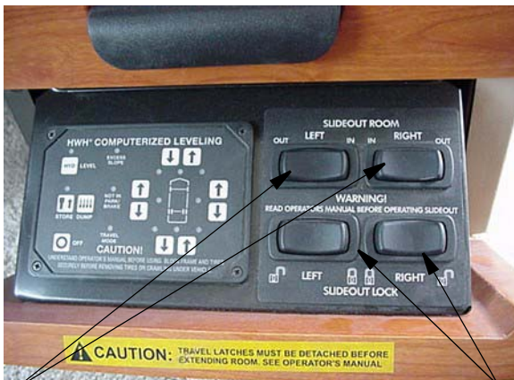
Front Slideout Control Switches
