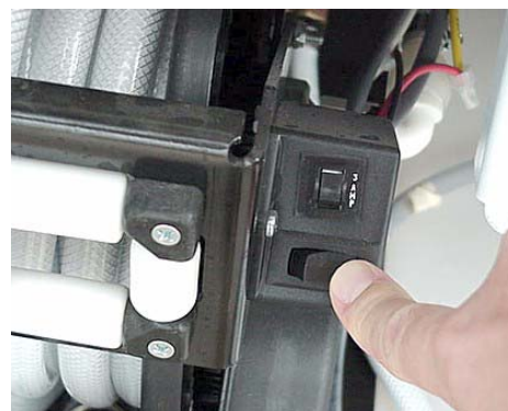
Press button and hold to retract optional water hose reel
