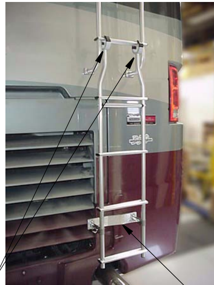
C-Brackets Bumper Support Ladder Extension (typical)
