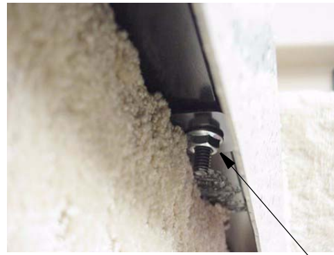
Hydraulic Pump Access – remove nut from bolt on underside of step and lift off step
