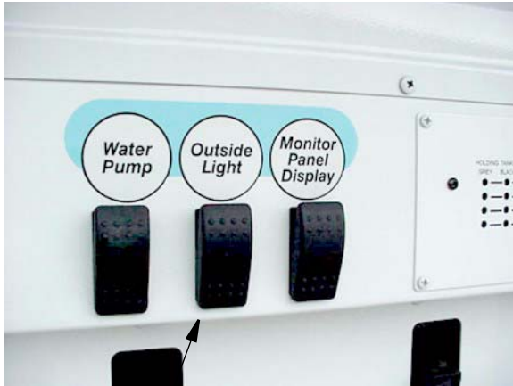
Utility Light Switch
