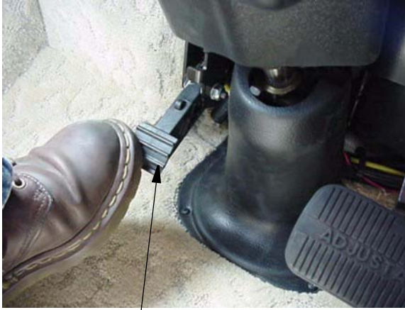
Press pedal to adjust steering wheel tilt or telescope
