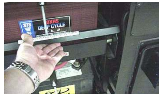
Lift Battery Tray Retainer Latches
