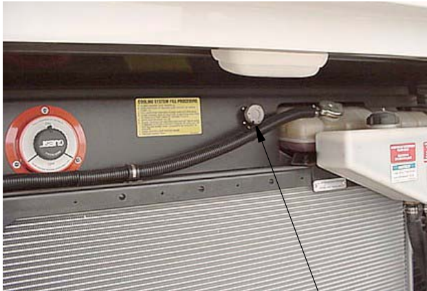
Diagnostic plug on rear engine compartment shroud
