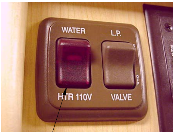
Electric Water Heater Switch (Typical)
