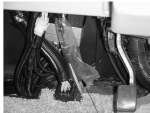
CB Wires (in plastic sheath)
