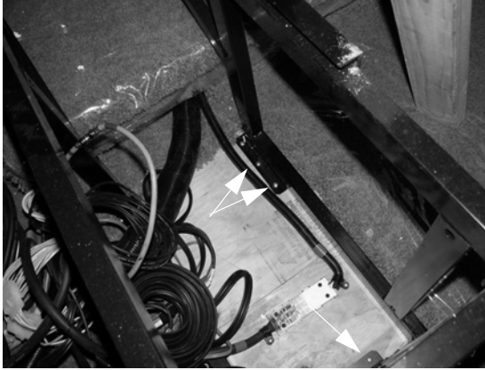
Steel Frame Screw Locations -Typical View
