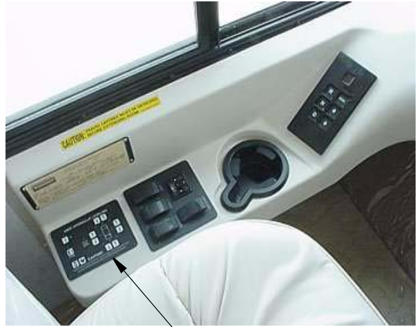
Leveling System Control Panel
