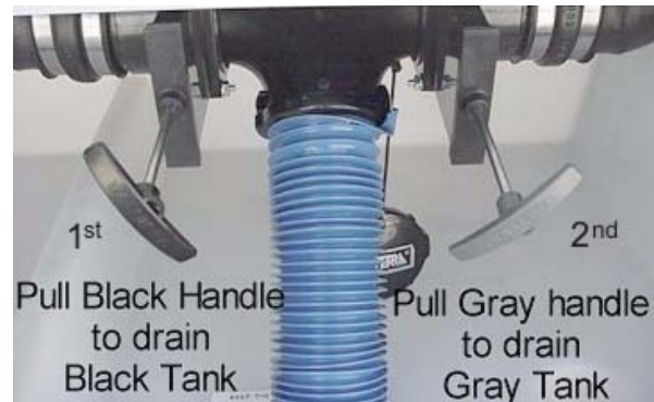
Holding Tank Valves (Typical)
