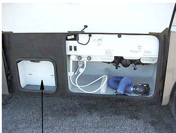
Water drain valves located behind access panel
