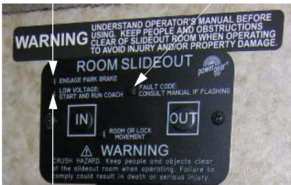
Low Voltage Indicator
