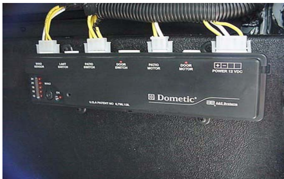
Awning Control Box (located in exterior compartment)
