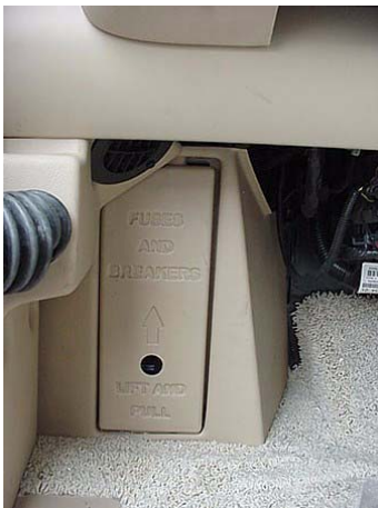
Automotive Fuse/Breaker Panel (Located beneath left end of dash)
