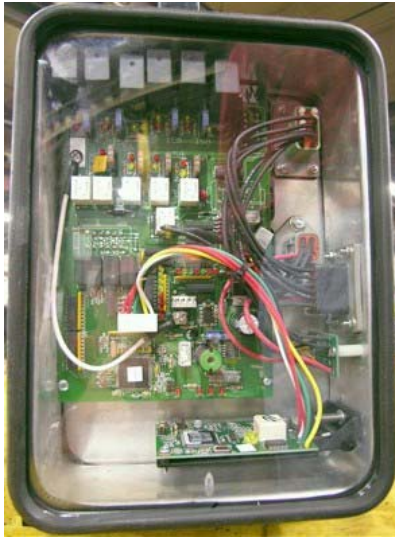
Hydraulic System Control Box (on pump beneath chassis near LH or RH front tire)
