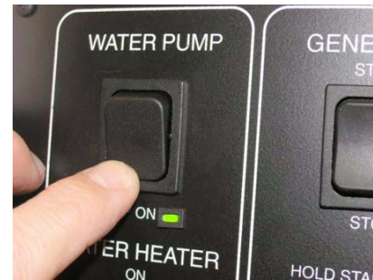
Water Pump Switch
